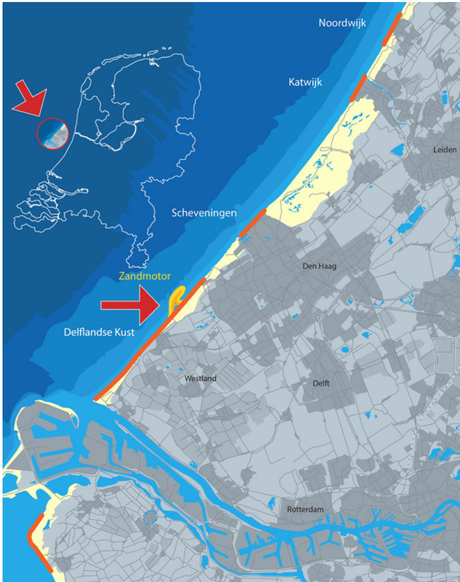
Fig. 4 The Delfland Sand Engine. The red lines indicate ‘weak links’ in the coastal protection system; the yellow areas represent dunes. The location of the Sand Engine ( Zandmotor in Dutch) was chosen near one of the weak links in the 15 km stretch of coast between the entrances to the harbours of Rotterdam and Scheveningen
